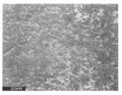
Figure 3: Isotropically superfinished surface showing the elimination of machining marks and distressed material zones
