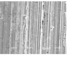
Figure 2: SEM image of a machined surface showing machining marks and distressed material zones
