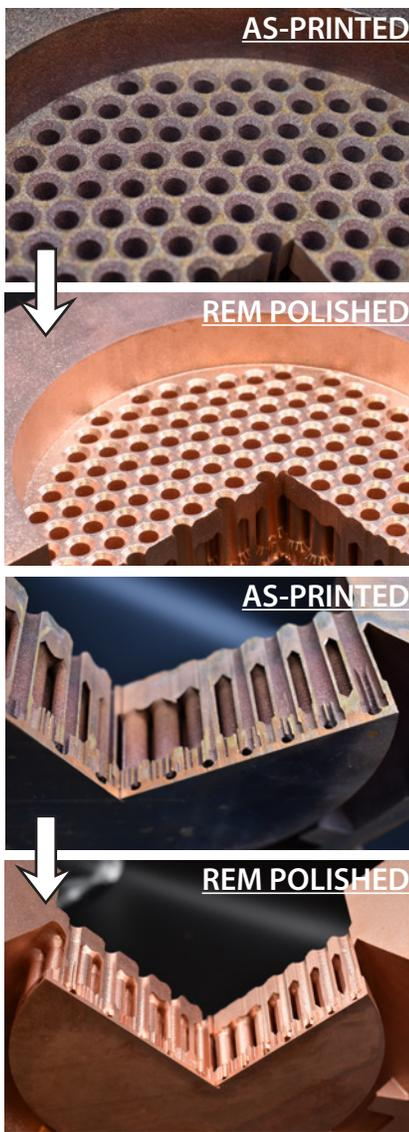
Copper is an important material to the rocket propulsion industry due to its high thermal conductivity. Thrust Chamber Assemblies (TCA's) and associated components such as fuel injectors and heat exchangers are excellent component applications for copper alloys.
