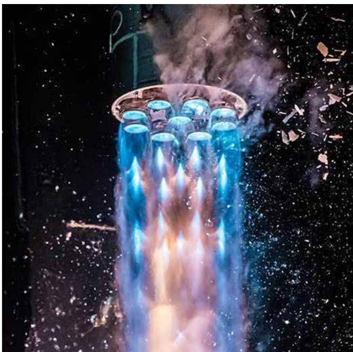
Figure 2: Launch of Relativity Space's Terran Rocket using additively manufactured copper alloy thrust chamber assemblies. (Courtesy: Relativity Space) [5]
