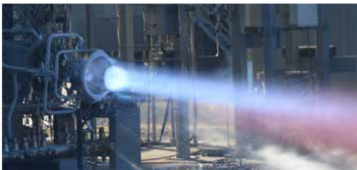
Figure 1: Hot fire testing of an additively manufactured rocket engine with a GRCop-42 combustion chamber and internal cooling channels as a part of the RAMPT project. (Courtesy: NASA MSFC) [4]
