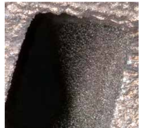
Figure 5: PBF-LB/GRCop-42 as-printed internal channel surface (Courtesy: REM Surface Engineering)
