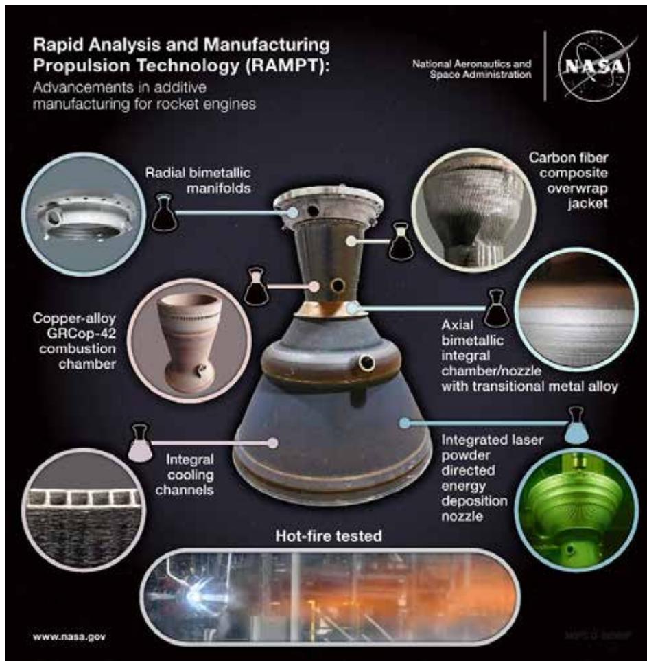
Figure 3: RAMPT Project summary graphic showing integral cooling channel application to the thrust chamber assembly. [6]
