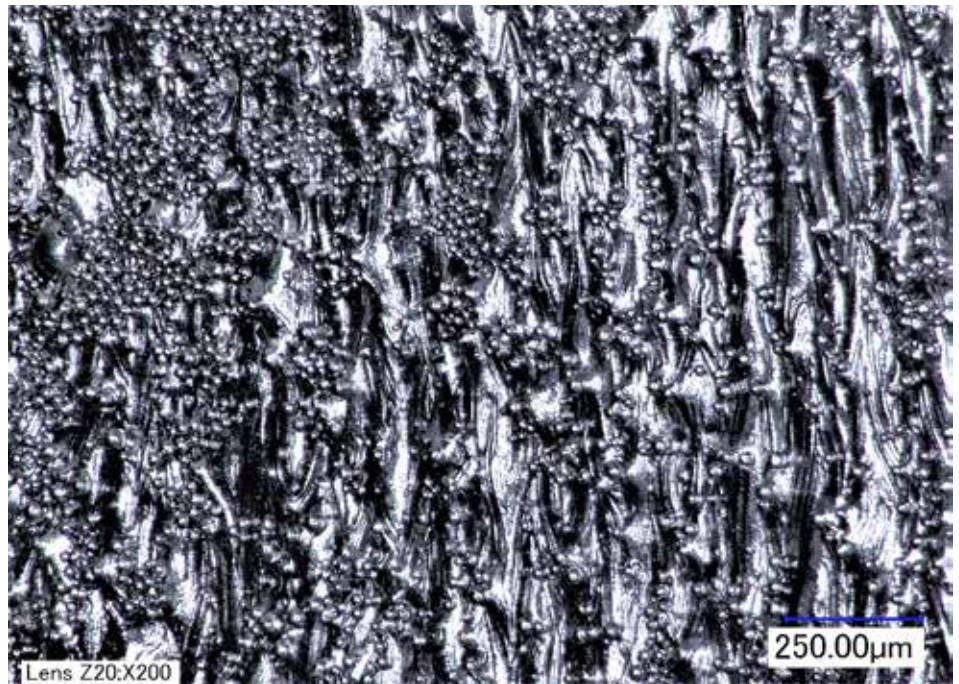
Figure 2: PBF-LB/Ti-6Al-4V surface showing high levels of texture and granularity (Courtesy: REM Surface Engineering)
