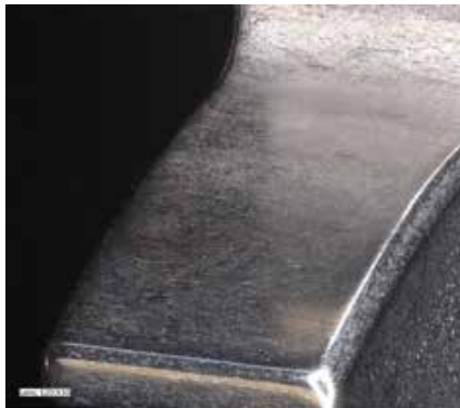
Figure 5: 30x magnification showing complete peening dimples removal after the second short rework cycle.
