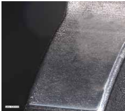
Figure 4: 30x image showing improved, but incomplete, peening texture removal following the first rework process.
