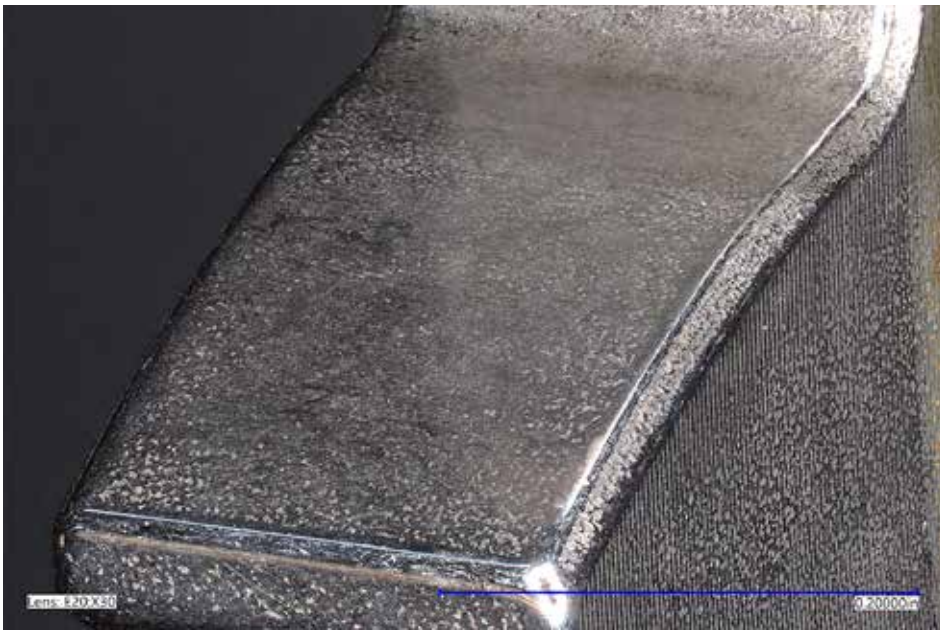
Figure 3: 30X image of tooth flank revealing hidden shot peen dimples after burnish step to remove the conversion coating.
