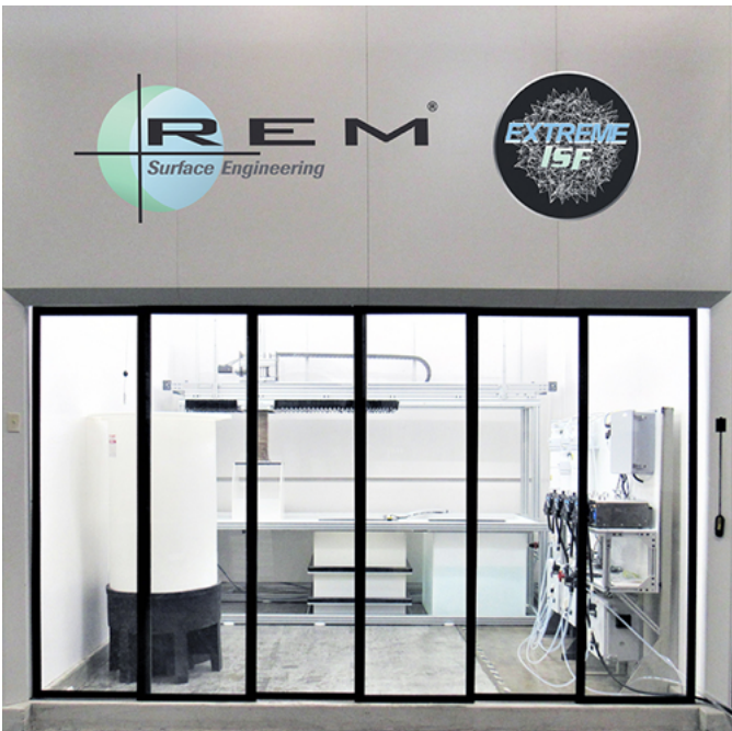
REM Surface Engineering already had experience finishing 3D-printed surfaces but had never worked with certain high-performance superalloys NASA needed for rocket engines. With the help of two SBIR contracts, the company designed and constructed this large-scale chemical polishing cell, where it polished NASA's superalloy nozzles. Today the company is ready to use the equipment for commercial clients. Credit: REM Surface Engineering
