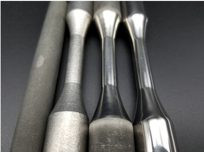
Building rocket parts using 3D printing is less expensive than traditional manufacturing methods and can facilitate complex shapes without joints. But the technique leaves rough surfaces (left) that could cause turbulence, corrosion, and accelerated wear if not perfectly polished (right). Credit: NASA
