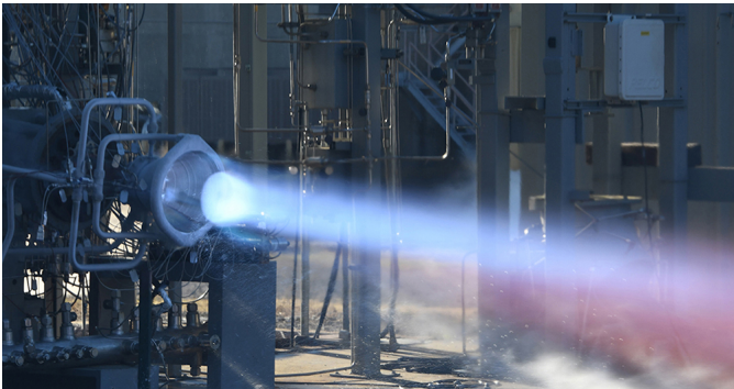
In this hot fire test at Marshall Space Flight Center, a nozzle printed from a NASA-developed superalloy metal is used inside the combustion chamber. The nozzle's surface was polished by Southington, Connecticut-based REM Surface Engineering, with a process and tools developed under SBIR funding from Marshall. Credit: NASA
