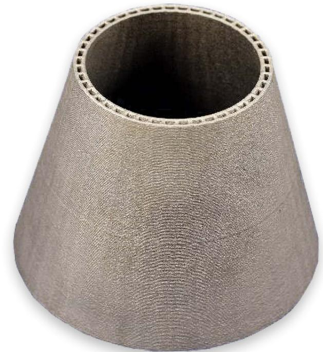
Fig. 6 Demonstrator component, BP-DED IN625 (Courtesy NASA MSFC)
