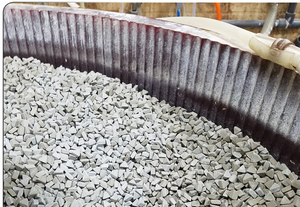
Ribbed liners are typically utilized in applications where flat parts are being processed or flat media must be used.
