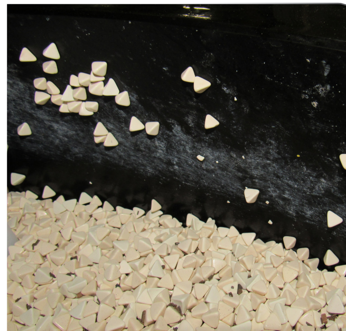
Media adhering to the inside wall of a vibratory bowl.
