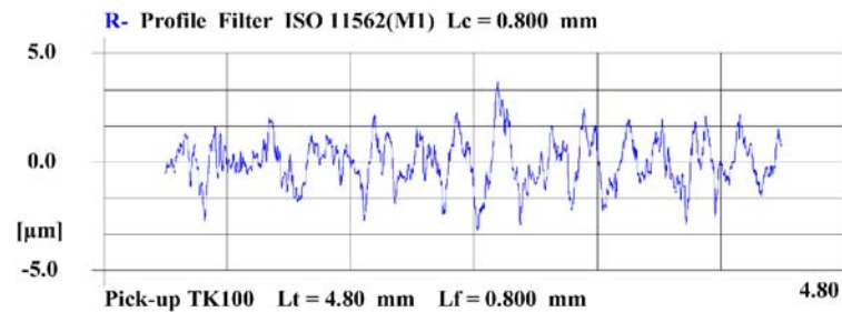
Figure 6a. Surface trace of a new ground low-speed stage pinion before superfinishing (2282)
