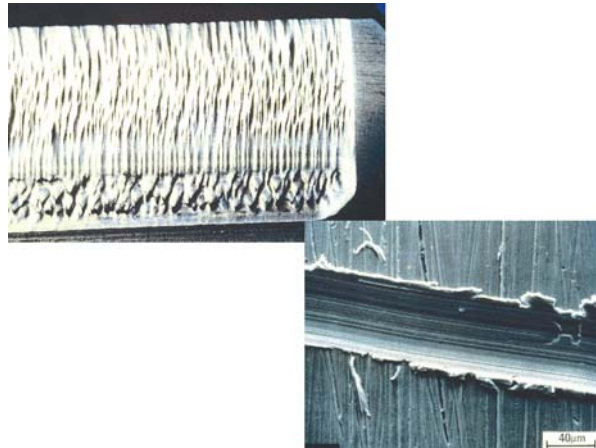
Figure 1b. Heavy abrasive wear on gear flank and a SEM image of trail left by an abrading particle [4]
