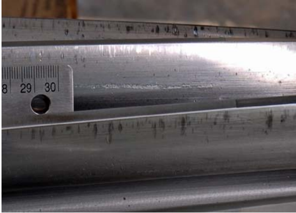
Figure 8a. Sun pinion gear with several modes of damage including hard line micropitting
