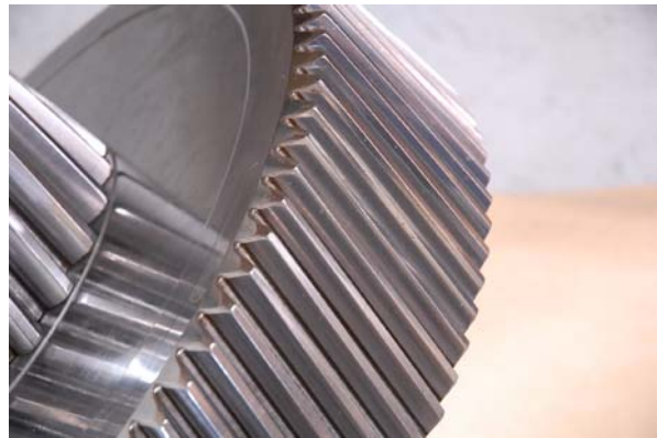
Figure 7a. Superfinished intermediate gear assembly (photo courtesy of Moventas)
