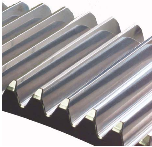
Figure 5: An image of a section of teeth from the third stage bull gear after Superfinishing. Note the reflections of the other teeth across each flank.
