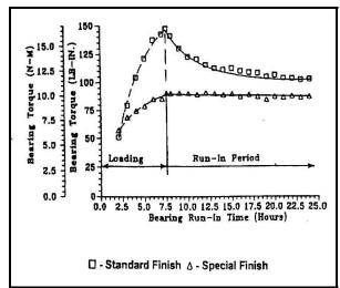
Graph 2; Shows the break-in period torque curve for a traditional ground surface and the Isotropic Superfinish (ISF).. Note the torque spike for the traditionally ground surface and the absence of a spike for the ISF.<sup>27,11</sup>
