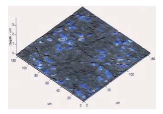
Photo 3; Shows a 3-dimensional, 20X magnified view of an ISF gear tooth. The  $R_a = is 1.5 \mu inches$ . The surface has been produced by chemically accelerated vibratory finishing. Note the elimination of the directional surface asperities (grind lines) when compared to Photo #2.
