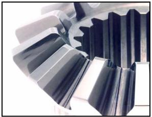
Photo 6; Shows a close-up of the teeth of the bevel gear as shown in Photo 1. The gear was processed using the described chemically accelerated vibratory finishing technique to generate the Isotropic Superfinish. The resultant surface has an is  $R_a$  of 1.5 µinches. Note when compared to Photo 1, that all grind line asperities have been removed.
