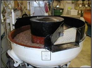
Photo 4; Shows a traditional vibratory bowl. Ideal for processing short stubby parts such as transmission gears, rocker arms and valve springs.
