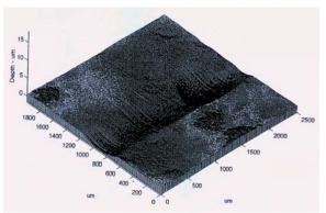
Photo 7; Shows the wear pattern produced in a blockon-ring evaluation<sup>6,7</sup> of the Isotropic Superfinish (ISF) steel block. The result of this evaluation
