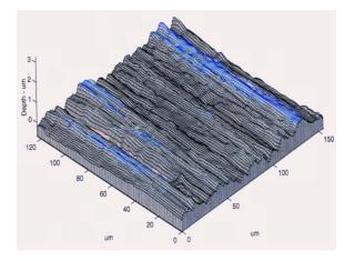
Photo 2; shows a 3-dimensional, 20X magnified view of the surface of a gear tooth that has been ground to a final surface finish of  $R_a = 35 \mu$ inches. Note the parallel rows of surface asperities corresponding to the directional pattern of the grinding operation.
