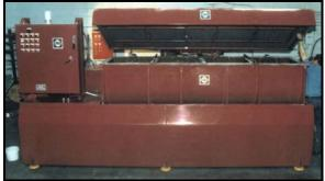
Photo 5; Shows a traditional vibratory tub. Ideal for processing long parts such as splines, camshafts, crankshafts and pinion shafts.
