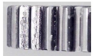
Photo 5; Shows gear tooth spalling caused by surface pit propagation. The gear shown was finished using traditional gear grinding techniques. Asperity peak contact during the gear break-in phase produced micro-pits, that with continued gear operation expanded and eventually coalesced into irregular craters over a significant area of the gear tooth.<sup>6</sup>
