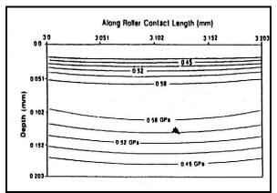
Graph 4; Shows a plot of the measured shear stress values of the Isotropic Superfinish tapered roller bearings along a 0.2 mm length of the tapered roller bearing's contact area.<sup>11</sup> Note that the high stress location is at a subsurface depth of 0.076 mm and that the surface stress values are < 0.45 GPa.
