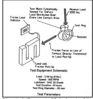
Schematic 1; Shows a simplified schematic of the block-on-ring apparatus.
