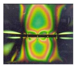
Figure 4: Image of the pressure peak caused by a hard particle in a contact zone.
