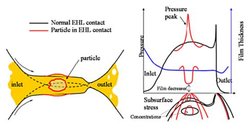
Figure 3: Schematic of a contact zone containing a hard metal particle and its resulting pressure peak.
