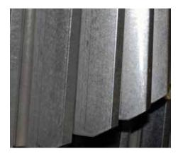
Figure 6: Closeup of the top planet after seven years showing no metal to metal contact pattern.
