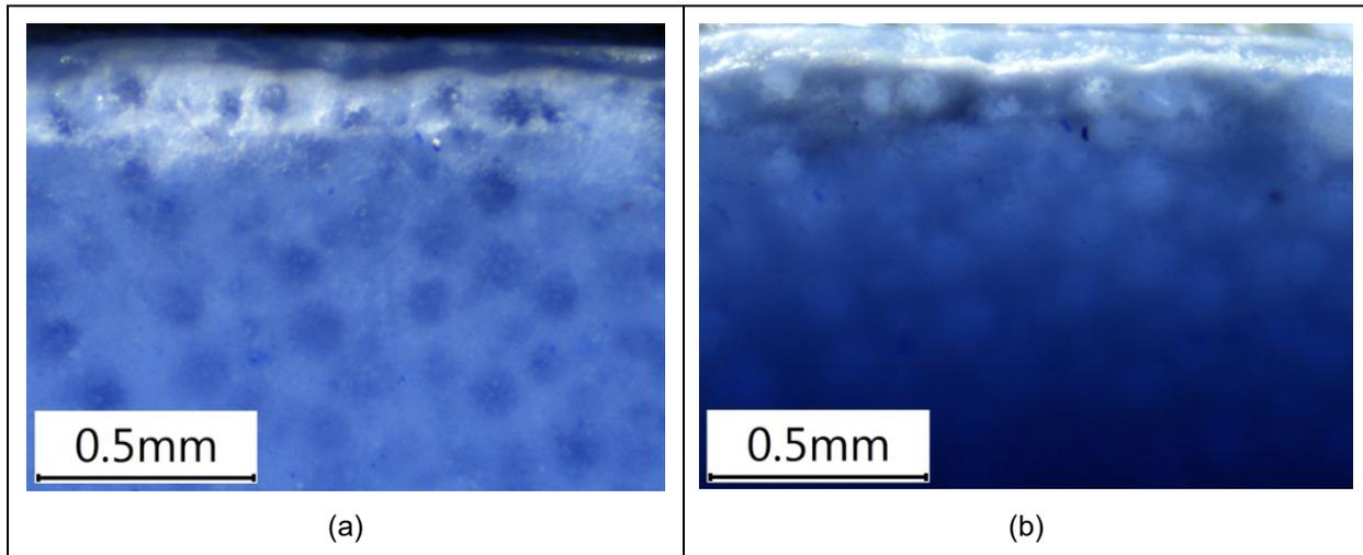
Figure 21 – Hard epoxy replica of ISF surface with (a) light source normal to surface shown and (b) light penetration into sample from side lighting
