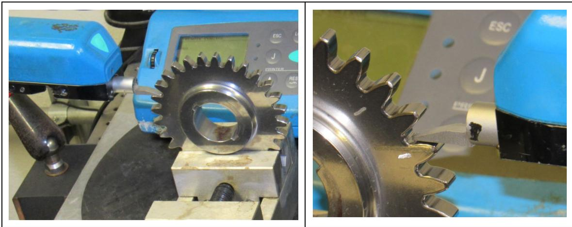
Figure 3 - Profilometer A, "shop floor" model
