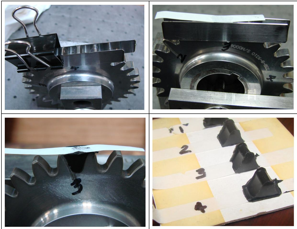
**Figure 1 - Silicon rubber replication process**
