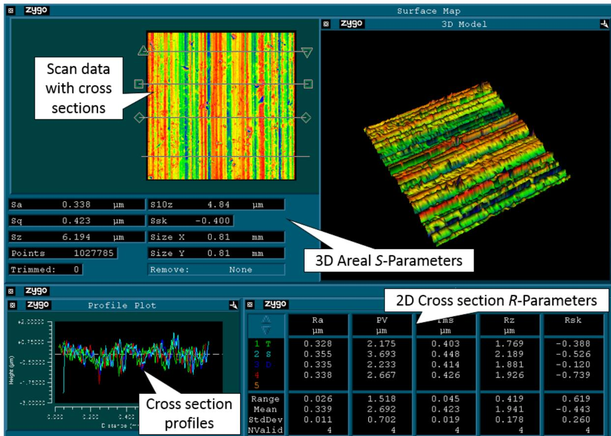
**Figure 6 - Processing of interferometry data**
