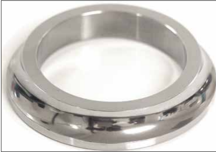
Figure 6: Example of an isotropic superfinish on a bearing race
